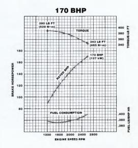
POWER OUTPUT guaranteed within 5% at rated ambient conditions. THIS RATING does not include power requirements for accessory and standard equipment.
